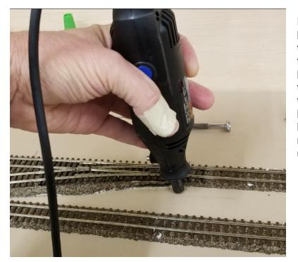
Replace the switch in its location, with the center of the throw-bar hole located over the pre-drilled hole. Drill three holes, two on either side of the throw bar and one along the centerline of the track behind the switch. These will be used to align the switch machine accurately underneath the layout.
