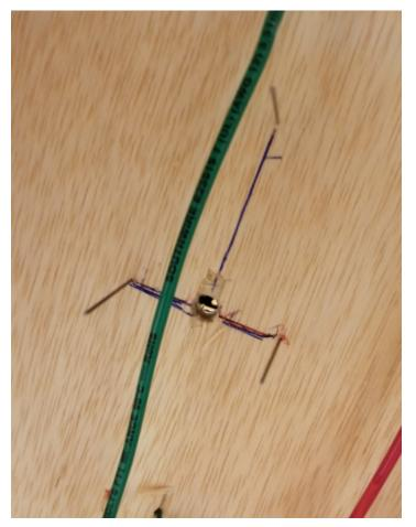
From below the layout, draw two lines, one from the center of the  $\frac{3}{8}$ inch hole to the flag behind the switch, and the other between the two flags on either side of the throw-bar through the center of the  $\frac{3}{8}$  inch hole.
