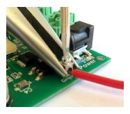
Hold pin with pliers while tightening to prevent twisting off connector.
